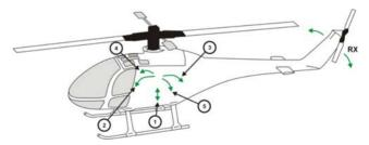
A helicopter with 4-point-control of swash plate (2 roll- und 2 pitch-servos). 1 = throttle. The gyro (tail rotor) is supplied directly by the receiver (5.2V) or via channel 6/1 of the DPSI (5.9V).
