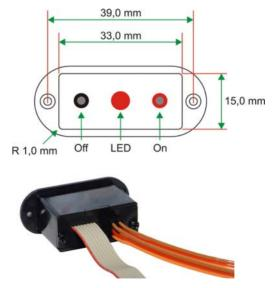
Rear side of the switch transmitter with connected battery controllers (optionally)
