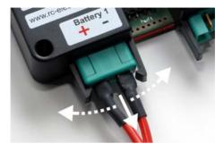
Removing the battery plugs from the DPSI RV Mini:
