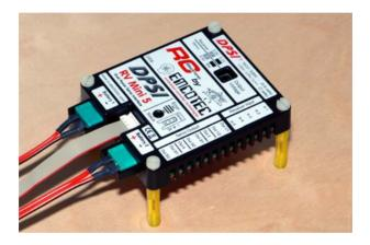
In general, always observe vibration free mounting including good air circulation. Vibration damping is especially important for the receiver because it is much more sensitive to mechanical stress than the **DPSI RV Mini**.
