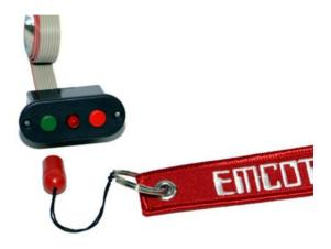
The central ultra bright LED in the switch actuator housing is lit when the **DPSI RV Mini** is powered. In case of errors (e.g. low voltage) or during programming, the LED indicates the states by different blink codes.
