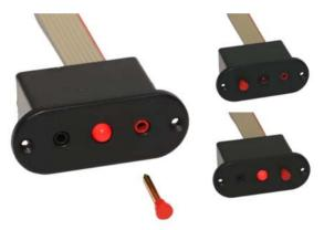
Of course, two pins must not be put into each of the sockets at the same time although this does not damage the **DPSI RV Mini**. In this case, the set would be turned off and the batteries would be discharged slowly with approx. 12mA. In the powered state the pin should always remain in the ON socket!
