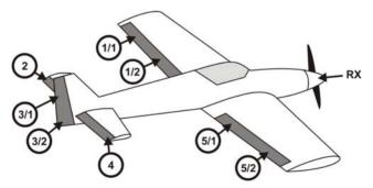
An acrobatic airplane with 2 servos per aileron and 2 servos for the yaw rudder. The throttle servo is directly connected to the receiver.
