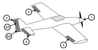
An acrobatic airplane with one servo per rudder, the yaw rudder is actuated by 2 servos.
