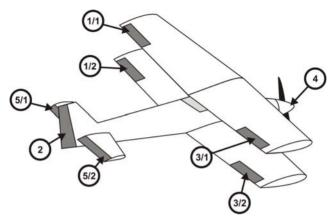
A biplane with 4 aileron servos, split elevator- and one yaw-rudder servo. The throttle servo may be directly connected to the receiver as an option.
