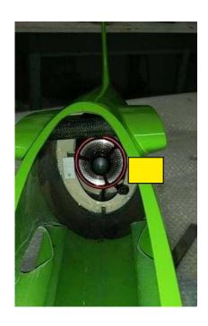
fuel tank: a special custom made fuel tank is supplied in the kit complete with tank cap and tank mounting rails
