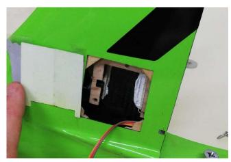
install elevator servo use one the supplied servo holder
