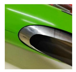
now you can apply the self adhesive alloy foil tape to protect fuselage from exhaust hot air
