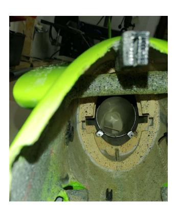
now you have to install the 3rd screw that keep the exhaust in position (may help making a small hole with a drill in the fuselage, exhaust will comewith hole already made ) inserting the small piece of high temperature resistant rubber between the exhaust and the fuselage to make installation easier we suggest you to shape the small piece of rubber with a bevel like in the picture.
