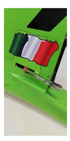
to install rudder servo use 2 or 3 of the supplied servo holder, depending on servo thickness, servo horn and control horn Check accurately before glueing permanently
