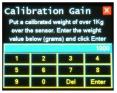
It is always recommended to calibrate all 3 sensors at the same time, so that all 3 are calibrated with same reference weight. Differences of calibration between sensors will cause errors in the measured weight and in the CG position. If all sensors are calibrated using same reference, even if the reference weight is of a non-exact value, the error will only be in the weight measure, but CG position will be correct.
