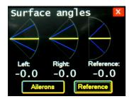
The graphic includes the current position of the surface and the maximum deflection positions, marked in BLUE lines. The current position line is YELLOW in color when the position of the surface is between minimum and maximum. The color will change to GREEN when the deflection is exactly as desired (+/-  $0,5^{\circ}$ ). If the deflection is excessive, then the line color changes to RED.
