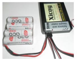
Connect a standard battery (not supplied) on the "Bat" input. Battery voltage could be from 5V to 9V.
