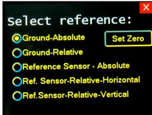
The Side Buttons allow selecting the reference for the measurements.
