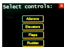
The left side one ("Ailerons" on picture) allows to select the surface to be measured. The BLUE lines on the graphic will be drawn accordingly to the data entered for this particular surface and the
