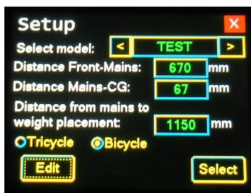
The unit can store the settings of up to 100 different models. Use the < and > buttons to change models. The model name (TEST in the picture) and the distances will be displayed.
