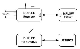
• Connection of the MFlow to the DUPLEX receiver via Expander
