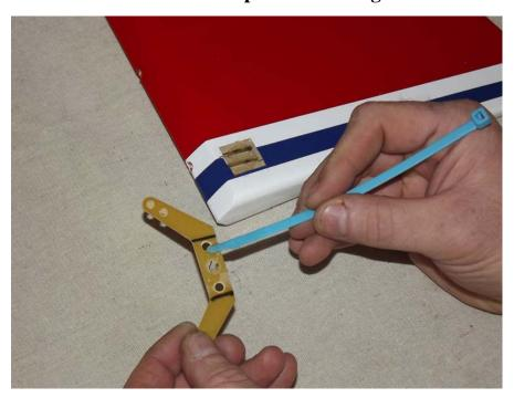
24. Slide the rudder horns back into their proper position. Clean the excess epoxy from the horns, and then install the base plates.
