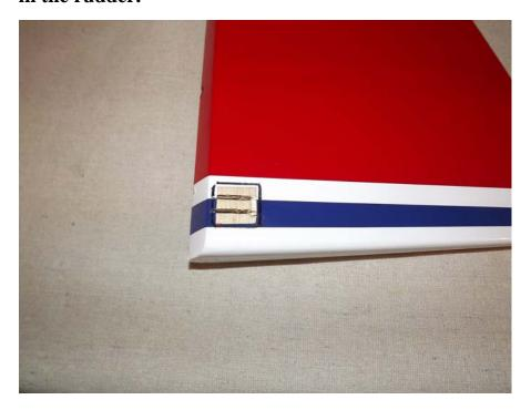
21. Before applying epoxy, measure the control horns to ensure they are centered properly and mark their location with a felt tipped marker. This will make it easy to reinstall control horns when epoxy is applied.
