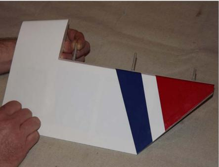
13. Now coat the other side of the hinges with epoxy and install the elevator into the stab, making sure the hinge pins are centered in the hinge gap. Don't forget to apply epoxy in the hinge holes on the stab before installing the stab to the elevator.
