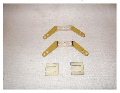
23. Mix a generous batch of epoxy and completely fill the two slots as well as the areas on control horns and base plate that will glue into the rudder.
