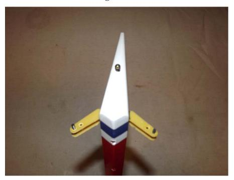
27. Next install the rudder hinges using the same procedure as with the Ailerons and Elevators.
