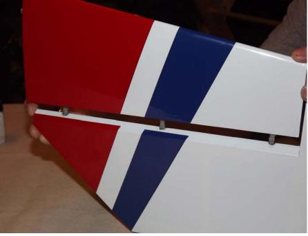
14. Use denatured alcohol and a cloth to remove all excess epoxy, especially on the hinge pin. Make sure you have full deflection in both directions – once satisfied with the results, set the surface aside to dry. After the hinges have dried thoroughly, pull on them to make sure they are properly installed. Repeat this process for the other stab/elevator half.
