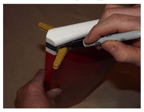
22. Scuff the middle of the horns that will go into the rudder as well as the base plates.
