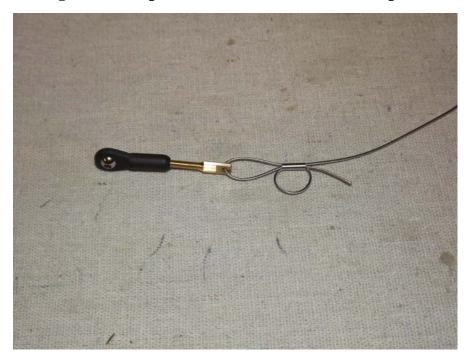
39. Insert the bare end of the cable into the slot in the rear of the fuselage and feed it forward into the canopy area. Make the same type of linkage as done previously. Electronically center the servo and secure the linkage at both ends with a 3mm bolt and nylon insert lock nut. Repeat for the other side.
