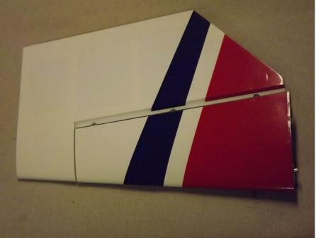
Note: Now is a good time to seal the hinge gap with a strip of Ultracote or Blenderm tape. Be sure to fully deflect the control surface when sealing the gap to allow for full deflection once the gap is sealed.
