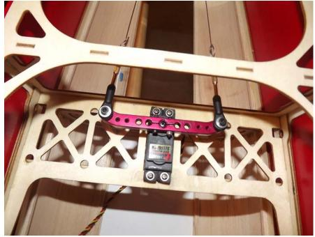
Note: When routing the pull-pull cables through the fuse, they should cross like an "X". Also, the tension on the wires should taut but not overly tightened.
