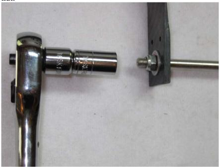
20. There is a pre-cut slot in the wheel pant to allow it to fit over the axle. You may need to open this slot with a rotary tool to allow it to slide into position over the axle. When satisfied with the position of the wheel pants, drill 2 holes through the plywood plate that is glued inside the pant at the location of the holes in the landing gear. Secure the pant in position with the provided 3mm bolts and blind nuts. Repeat this process for the remaining wheel pant.
