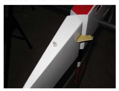
25. Slide the tiller arm into the ball link and secure the tailwheel assembly to the rear bottom of the fuselage with the supplied 3mm bolts inserted through the carbon tailwheel assembly and into the preinstalled blind nuts in the bottom of the fuselage.
