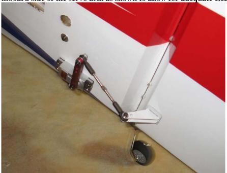
29. If using the pull-pull system you will want to mount the servo in the servo try under the canopy. There are locations for 2 servos here so it is possible to use servos ganged of a lesser torque value. No hardware is included for a tandem servo set-up. For proper geometry use the SWB 4.5" offset rudder arm or a similar unit.
