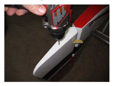
24. Glue the ball link into the bottom of the rudder using epoxy. Allow a small amount of epoxy to pool around the ball link shank for best results.
