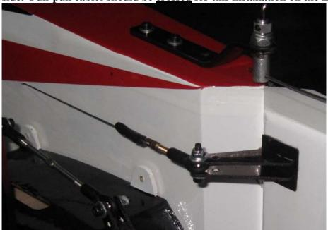
33. Slide both stab/elevator assemblies onto the carbon fiber mounting tube and secure with 2 3mm bolts inserted through a washer and the mounting tabs and into the corresponding blind nuts already installed in the fuselage. Be sure to use a drop of blue Loctite on all bolts!!!
