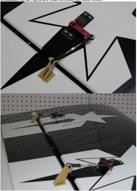
14. It is highly recommended that you use a servo programmer, Matchbox, Powerbox or power distribution unit to make sure both servos work in unison. We use the Hitec 7955s and 7950s in our aircraft in conjunction with the Hitec programmer and have been able to get the servos matched perfectly with very little current draw.
