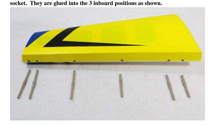
2. Install the control horns for the ailerons. \*\*\*PLEASE NOTE\*\*\* There are 2 different size control horns for the ailerons. The 2 longer sets are for the outboard aileron servos, the 2 shorter sets are for the inboard locations. Pay very close attention when separating and grouping the horns to be sure you are gluing the correct horns in the correct location! (Figure 2).
