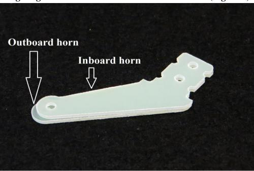
Insert the horns into the base plate and then temporarily install them in the aileron. Trace around the base plate with a fine tipped felt marker and then remove the horn and base plate. Use a sharp hobby knife to cut 2mm inside the line you marked and remove the covering. Scuff the bottom portion of the control horn that inserts into the hole in the control surface. Use epoxy to secure the control horns in place.
