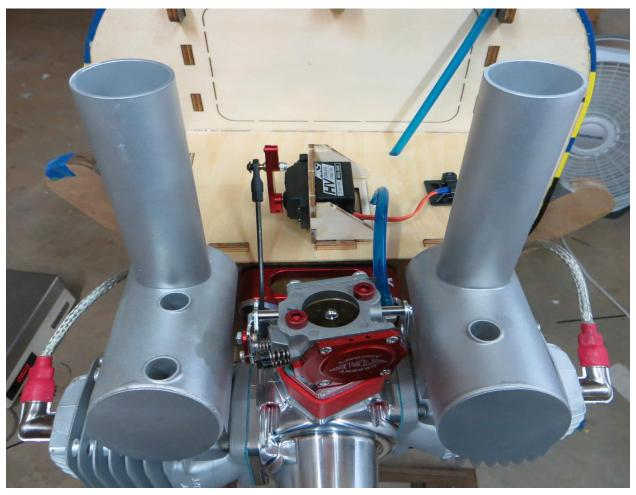
13. A set of engine baffles has been provided to duct air over the engine cylinders. These will need to be trimmed to fit your chosen engine. Glue in place with Goop or epoxy.
