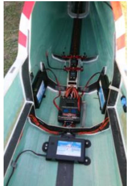
RC-installation for DA200. If you intend to fly more pattern, you can install the ignition battery a bit closer to the front.
