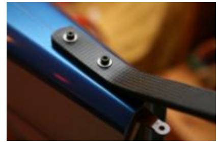
Our carbon tailwheel installed under the fuselage with two M4x20mm Screws.
