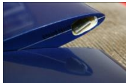
Glue 20 grams of lead inside the mass-balance area in order to static-balance the elevators
