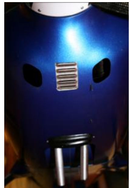
The canister exhausts and the cutouts in the cowling (DA200)
