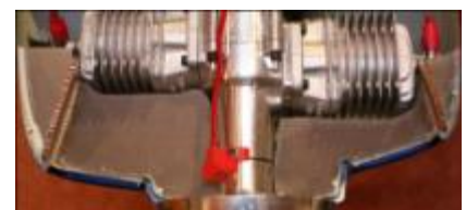
The baffle plate inside the cowling (DA170)
