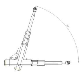
To change the bracket point is necessary extract the socket screws installed at both fork sides. Both socket screws are opposite, to be fastened, after tight at the same time with two allen keys. **To secure this is important tight both socket screws with a mínimum torque**. This step, will liberate the actuator spin around this "axle".
