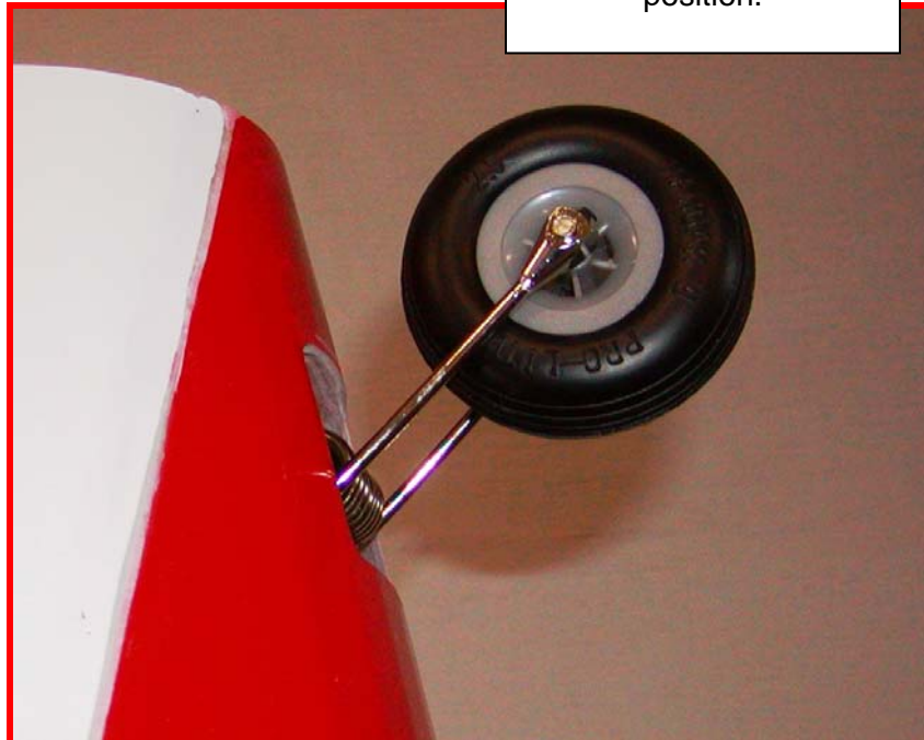
The Gee Bee now comes with a fiberglass tailwheel fairing. The fairing is secured using the TW axle. The axle is secured using the set screws at the bottom of each leg.
