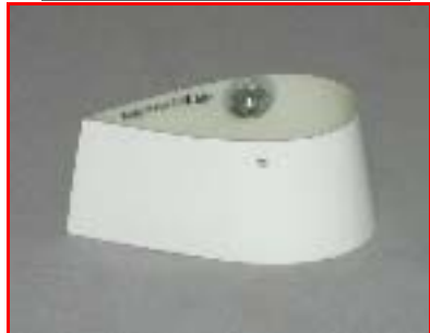
The Gee Bee now comes with a fiberglass tailwheel fairing. The fairing is secured using the TW axle. The axle is secured using the set screws at the bottom of each leg.
