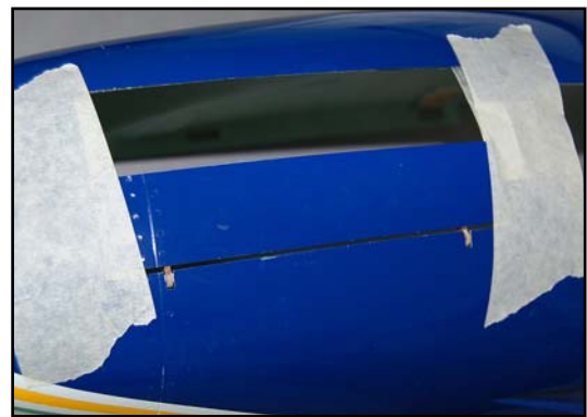
(below) File 4 slots in the cowl to match the positions of the phenolic plates.
