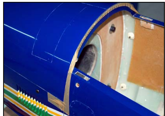
(below) Apply a thick bead of silicone to cowl and bolt in place until cured.
