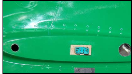
(above) Multiplex connector mounted in plywood plate, glued into stab root for elevator servo cable.
