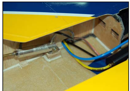
(below) Cylinder installed, and all air tubes and flap servo cable routed thru' the slot in the spar/balsa shear web.
