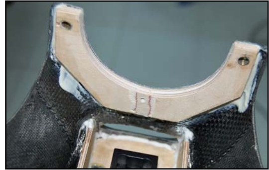
(above) For JetCat, make sure that the bottom engine mount clears the plywood surface by sanding a small groove. (below) Glue the inlet duct to the carbon mount, and trim the end flush. Glue on split silicone tube to minimise any gap between the duct and turbine.
