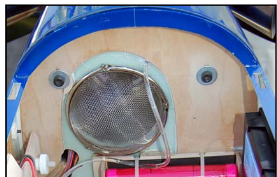
(above) For the JetCat it is important to fit a FOD-guard to make sure no small items are sucked in from the fuselage. (below) Completed air inlet louvre secured in with 6 sheetmetal screws.
