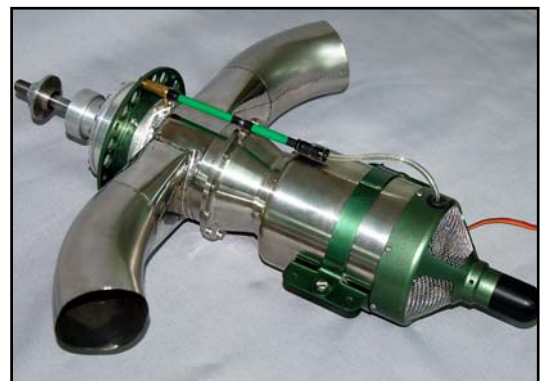
(above) Wren MW54 turboprop, showing vertical front mounting ring for the 2nd stage turbine & mounting strap for the core (rear) turbine. The exhaust outlets are integral part of the motor.
