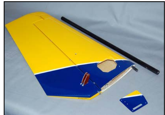
(above) Horizontal stabiliser parts.
