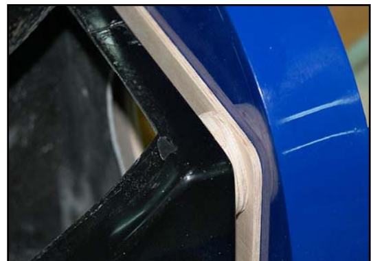
(below) For the Wren only you need to use 2 milled plywood discs in each corner of the firewall for correct spacing.
