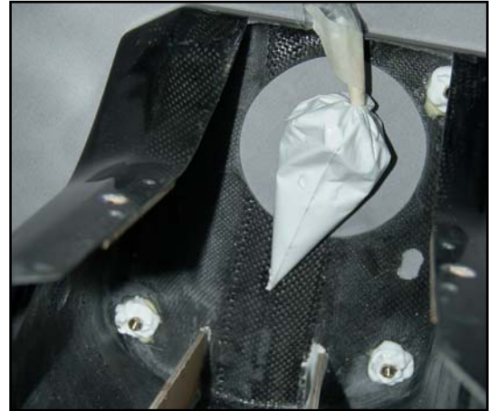
(above) M6 T-nuts are glued inside the carbon mount with a thick epoxy and microballoon mixture.
