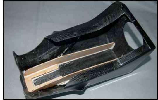
(above) The carbon motor mount is trimmed, and the plywood parts for the nose gear unit are factory-installed.
