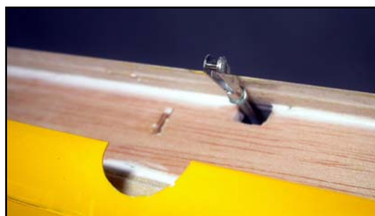
(bottom) Use a long 2mm drill to make the pilot holes in the rib for the \varnothing 2.9 \times 16 mm sheetmetal screws.
