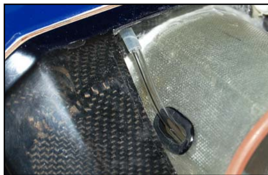
(below) Protect all fuel, gas and electrical services where they pass thru' any composite or wood parts
