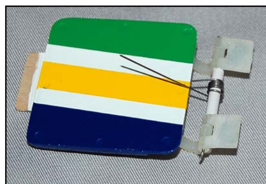
(above) Detail of the access hatch, with assembled offset hinges and spring - viewed from the outside.
