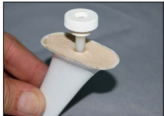
(below) Fuselage antenna's are simply mounted with M6 plastic bolt and nut.
