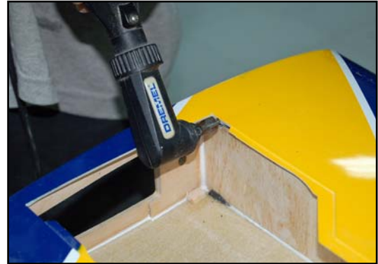
(above) A 90 degree attachment makes it easier to drill the hole for the front hinge tube.
