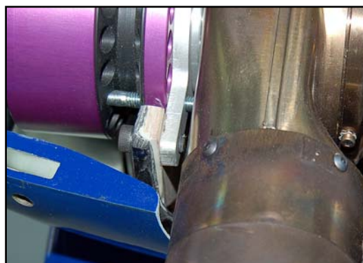
(below) Close-up view of one of the brass tubes glued into the front mount.
