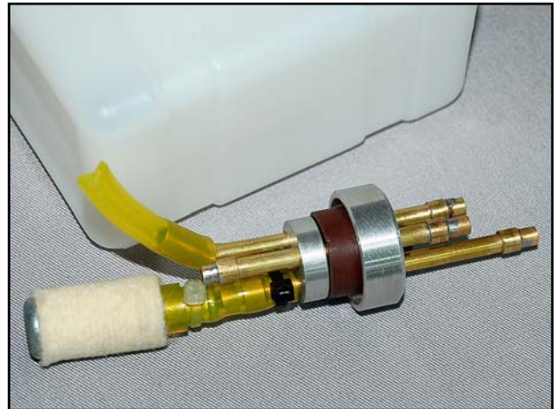
(above) The hopper tank has a 3-tube set-up, with the extra tube used for filling the fuel system. Make sure that the felt clunk is fixed as close to the 3-D centre of the tank as possible. (below) The rear tank and hopper tank mounts are assembled as shown here.
