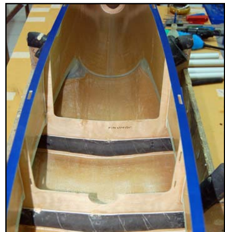
(below) All main structural bulkheads are factory-installed.
