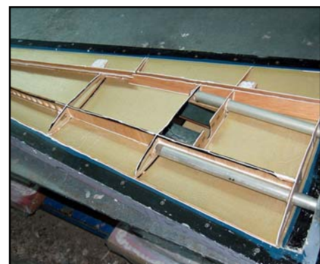
(top) Dual 30mm alloy wing tubes give excellent structural integrity.
