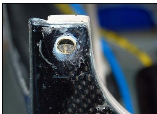
(below) Close-up view of one of the brass tubes glued into the front mount.
