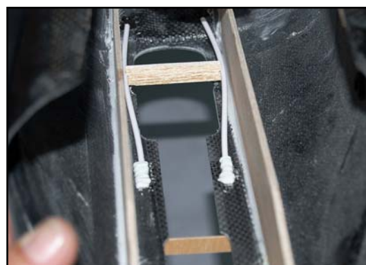
(above) The slots for the steering tubes should be about 20mm long, & 8mm away from the milled slot for the oleo. (below) Scrap balsa holds tubes apart while glue dries for wheel clearance.
