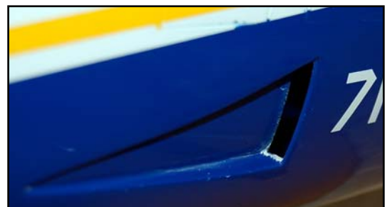
(above) You can mill out the vents in the cowling to provide extra cooling airflow.
