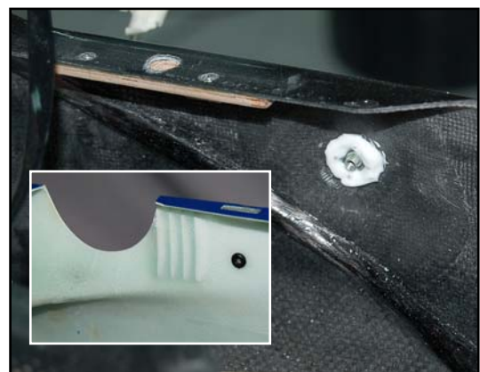
(inset) Half a small rubber grommet is glued to cowl with CA to act as spacer.
