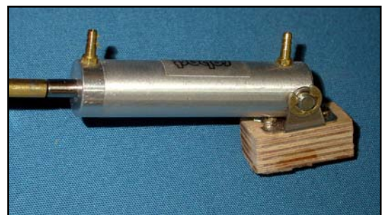
(below) Door cylinder fixed to mounting block with 2 small sheetmetal screws.
