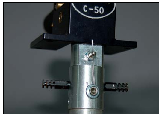
(above) The noseleg incorporates a small music wire that locates in an eye in the trunion block to keep it centred during retraction and extension.
