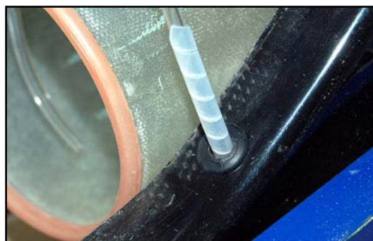
(below) You will need to drill holes in the plywood firewall and the back of the carbon motor mount for the tubes and electrical connections to the turbine, and also for the air tubes and steering cables for the nosegear.
