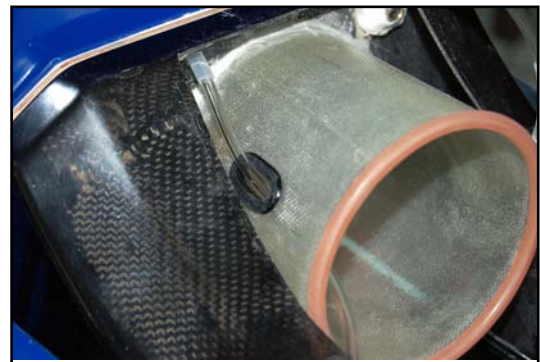
(above) For JetCat, make sure that the bottom engine mount clears the plywood surface by sanding a small groove. (below) Glue the inlet duct to the carbon mount, and trim the end flush. Glue on split silicone tube to minimise any gap between the duct and turbine.
