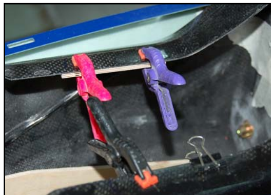
(above) Glue plywood strips under the carbon flanges for the core mount strap T-nuts, using epoxy.
