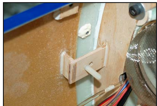
The Turbine/ECU board is secured with a plastic bolt & nut, glued into the milled parts included. The back has tabs that fit into slots in the adjacent bulkhead.
