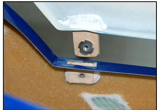
(above/below) The canopy frame fixings are completed at the factory for you.
