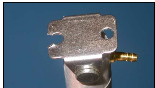
(above) Slot the inner hole in the door cylinder brackets.
