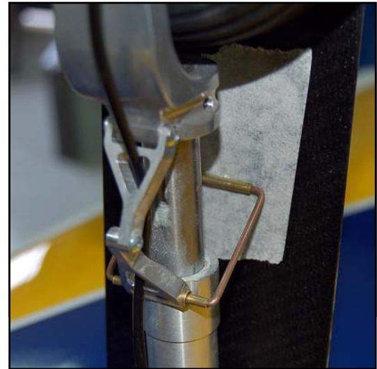
(above) Use masking tape on door to check for exact position of brass tube. No bend made for fine adjustment yet. (below) Brass tube on door is approx. 20mm above tube in scissor link. Adjust side bends for perfect closing.
