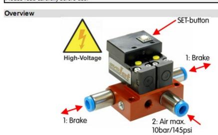
The evoJet **PRO-**Proportional – brake valve is made for wheel-brakes using compressed air. For a scale-like and controlled braking the valve uses proportional air dosage. A double working valve technique (fill or drain) needs just a minimum amount of compressed air (low loss).
