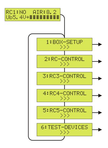
To leave the SETUP menu and to return to the BOX status display, press the SET key for more than 2 seconds (ESC). In the following, the individual submenus of the SETUP menu are described.
