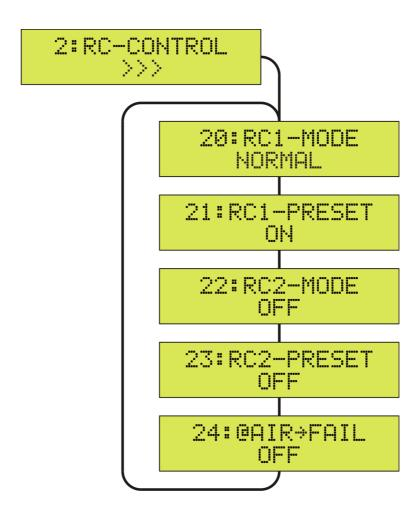
To leave the 2:RC2-CONTROL menu and to return to the SETUP menu, press the SET key for more than 2 seconds (ESC).
