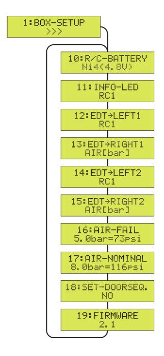
To leave the 1:BOX-SETUP menu and to return to the SETUP menu, press the SET key for more than 2 seconds (ESC).
