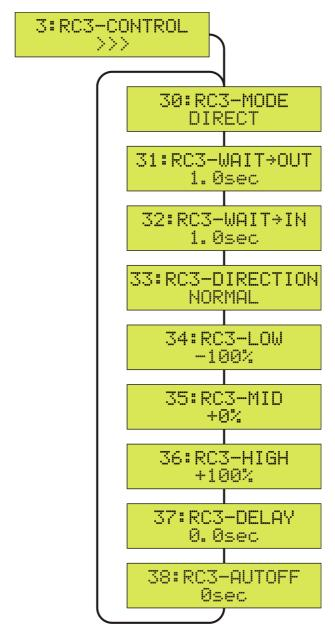
To leave the 3:RC3/4/5-CONTROL menu and to return to the SETUP menu, press the SET key for more than 2 seconds (ESC).
