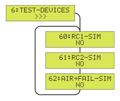
To leave the 6:TEST-DEVICES menu and to return to the SETUP menu, press the SET key for more than 2 seconds (ESC).
