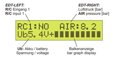
**EDT-LEFT** and **EDT-RIGHT** are configurable function displays for operating parameters. In the BOX-SETUP menu, you can choose what should be displayed in the *LEFT* and *RIGHT* areas.
