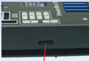
Socket for Multiplex telemetry MSB Also for Futaba and Hott when available This socket is also used for software updates
