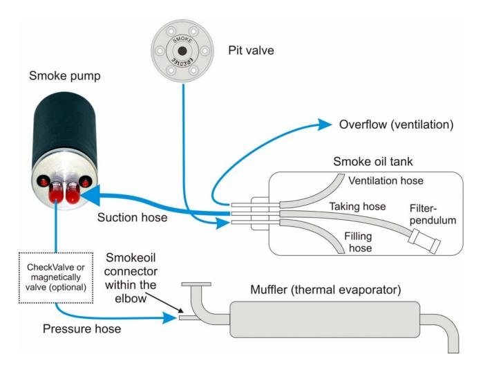
The **PowerSmoke 740 HV** has an integrated valve and can therefore be even positioned lower than the tank.
