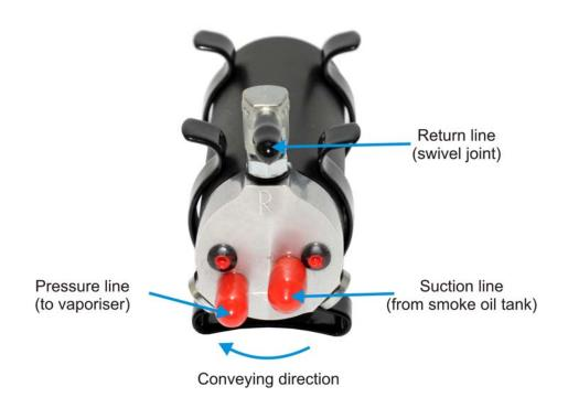
Flow direction is marked by an arrow. The "R" marked connector (swing fixture) is to be routed back to the tank. Back flow is approx. 35ml/min. In order not to install a separate connector to the tank, a delivered T-piece can be looped into the tanking hose. Here, the back flow is to be connected.
