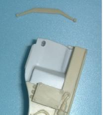
Glue with CA the plastic part at the rear of the ejector seat.
