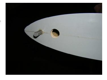
Make a 5 mm corresponding hole in the fuselage for the electric wire
