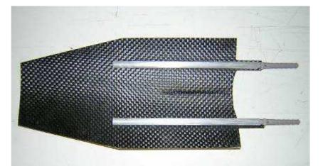
Glue the 2 Robart hinges in the tube with epoxy. Bend the hinges at 90° to be sure they are parallel
