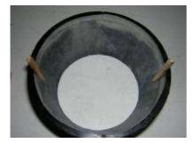
Screw the tailpipe with 2 x 2mm parker screws to secure the wood pins
