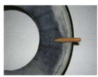
Glue with CA a 6 mm wood pins on 2 opposite sides of the exhaust cone
