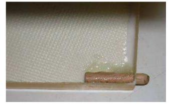
Glue the wood pin with CA in the hatch Glue the wood pin with CA in the hatch Drill the corresponding hole in the front fuselage
