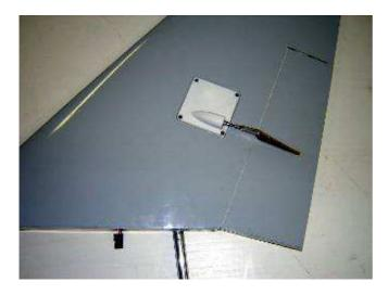
Cut a slot in the control surface for the fiber control horn
