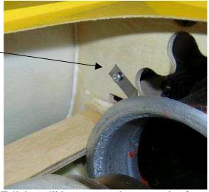
Tailpipe will be screw on the rear engine frame with  $2 \times 3$  mm diameter parker screws .
