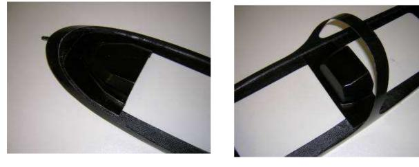
Gluing the clear canopy : Put the clear canopy inside the canopy frame. Hold it with paper tape Apply some ZAP canopy inside the frame between the clear canopy and the fiber parts Let in dry 24 hours
