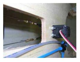
If necessary, add 2 soft springs or rubber bands to extand the wire when the front gear retract
