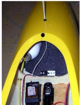
Gear valves, air tank, batterie, antenae
