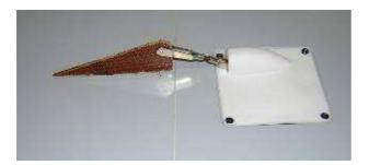
Cut a slot in the control surface for the fiber control horn Glue with fast epoxy the control horn Connect two 2 mm link with M2 threaded rod Screw the servo cover with the 4 parker screws Connect the servo with the control horn Apply thread lock.
