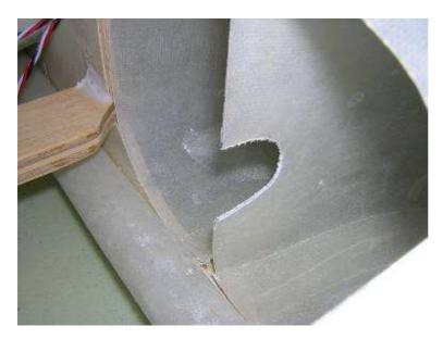
Adjust the position of the engine / beginning of the exhaust tube The engine must be screw with 4 times 3x20 mm parker screw to the rear position. Secure all electric wire and fuel tubing in front of the engine in the fuselage
