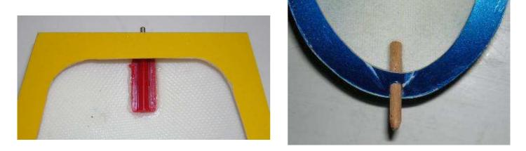
Glue the hatch latch with CA. Take care to not glue the metalic part Fit the hatch on the fuselage and draw the corresponding hole Drill the 3 mm hole in the fuselage
