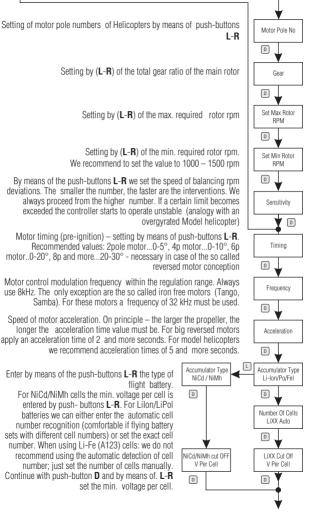
Information about the preset cut off voltage. With NiCd/NiMh cells or when setting the automatic detection for Lilon/LiPol cells this value results of the actual voltage of the connected flight batteries.
